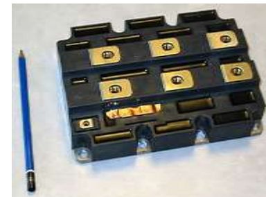
IGBT module (contains IGBTs and diodes)
